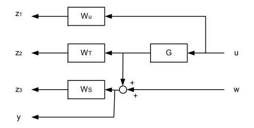
$z_{1} = W_{u}u$   $z_{2} = W_{T}Gu$   $z_{3} = W_{S}(Gu + w)$  y = Gu + w
