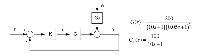
Command tracking + disturbance rejection problem Both demands are difficult to meet simultaneously (trade-off in control design)
