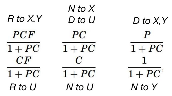
Feedback can be designed to deal with disturbances, feedforward response to reference changes!
