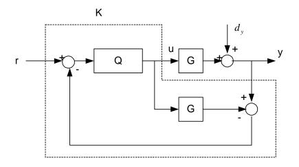
Note that in addition to the reference r a disturbance signal  $d_y$  is modelled to enter at the output of the process. By using the IMC design discussed in the lectures analyse the response to step inputs at r and  $d_y$ .
