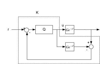
But what if the process G is unstable? Look at the previous problem, in which it was shown that the closed loop system is internally unstable, if Q or G is unstable. Because the Smith predictor structure was above shown to be equivalent to the *IMC*-structure, the closed loop is inevitably (internally) unstable, if the process is unstable.
