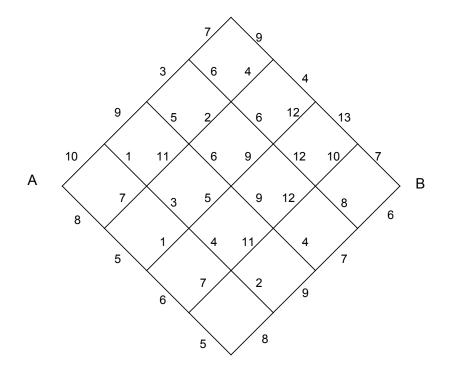
**Solution.** Use dynamic programming and the principle of optimality. Start from the end point B and mark to each state (node) the optimal cost and optimal control.
