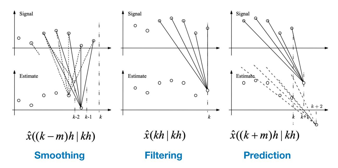
• In LQG control, the Kalman filter is used as a predictor.
