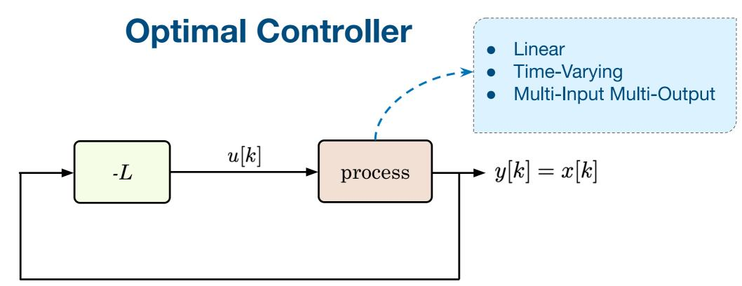
• LQR optimal control, with the gain to change over time based on the cost
