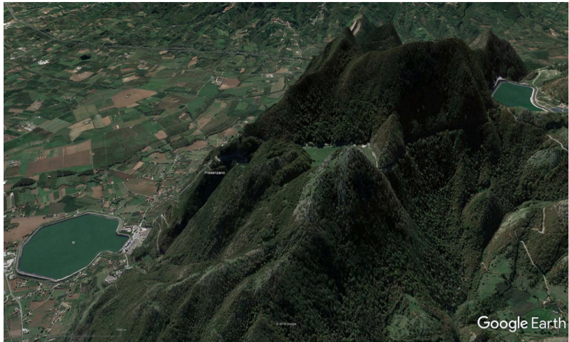
Figure 10. Google Earth synthetic image of a Gigawatt-rated off-river PHEs site at Presenzano in Italy, showing the two reservoirs (upper right and lower left) with a head of 500 m (vertical scale exaggerated). Map data ©2021 Google.
