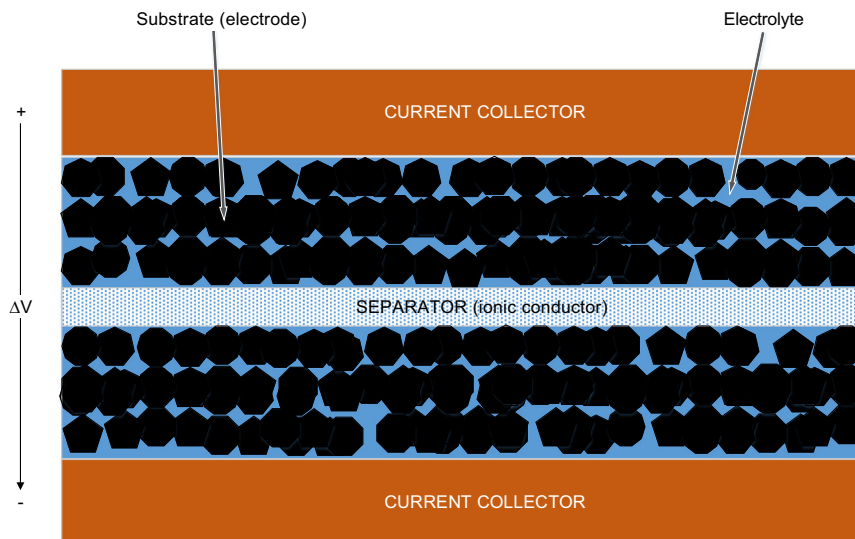
Fig. 4. Symmetric supercapacitor schematic diagram.
