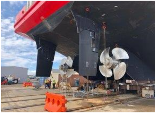
Figure 53. Twin rudder arrangement and 54. Ice knife implementation (Traficom, 2019)
