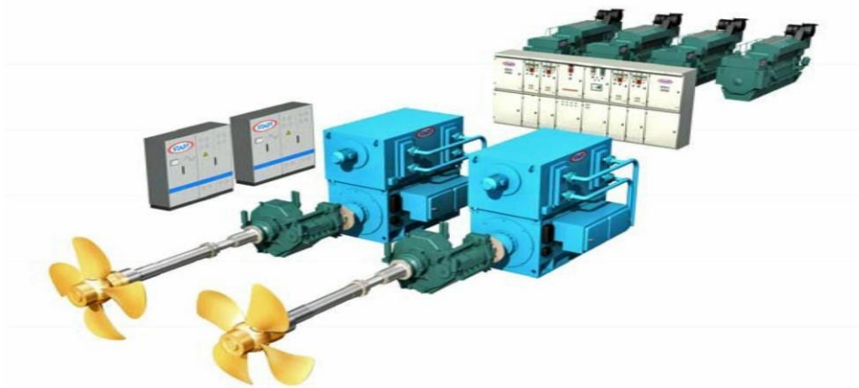
Figure 34 Example of Diesel-electric propulsion system (Ocean Time Marine, 2020)
