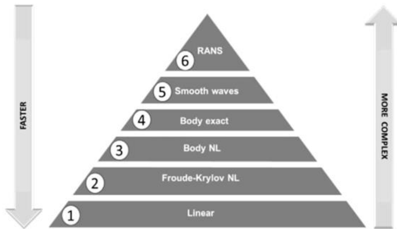
Figure 13-1 Level of idealization for forward speed hydrodynamic solutions. Figure from course notes.
