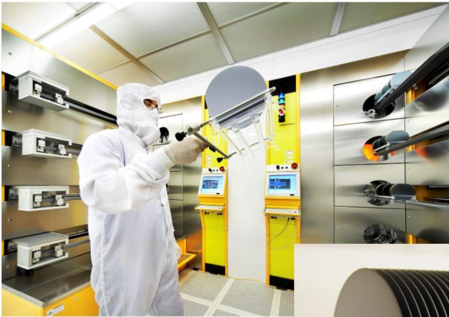
Micronova cleanroom, CVD (and thermal oxidation tubes).
