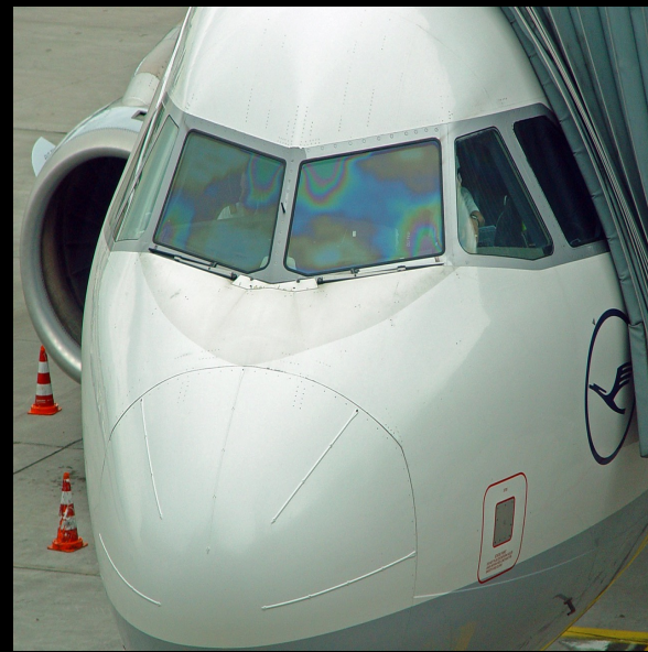
Indium Tin Oxide, ITO: Defrosting coating
