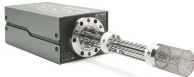
SRS RGA100 Residual Gas Analyzer
