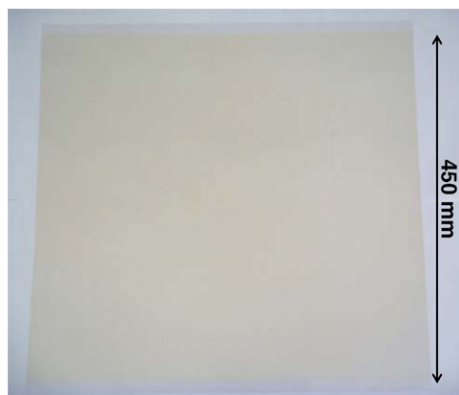
Fig. 9. The flat-type CVD equipment uniformly coats AP-DLC films with a size of 450 mm × 450 mm.
