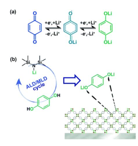
**Fig. 1** (a) The redox scheme of p-benzoquinone. (b) The ALD/MLD process for the Li<sub>2</sub>Q thin films.
