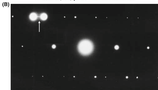
FIGURE 17.8. (A) Schematic of twin and (B) DP with a streak (arrowed) normal to the twin plane. Note that s=0 for the two bright diffracted spots.
