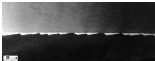
FIGURE 29.9. Diffuse-scatter DF image of a glassy material at a GB in a bicrystal of \text{Al}_2\text{O}_3 .
