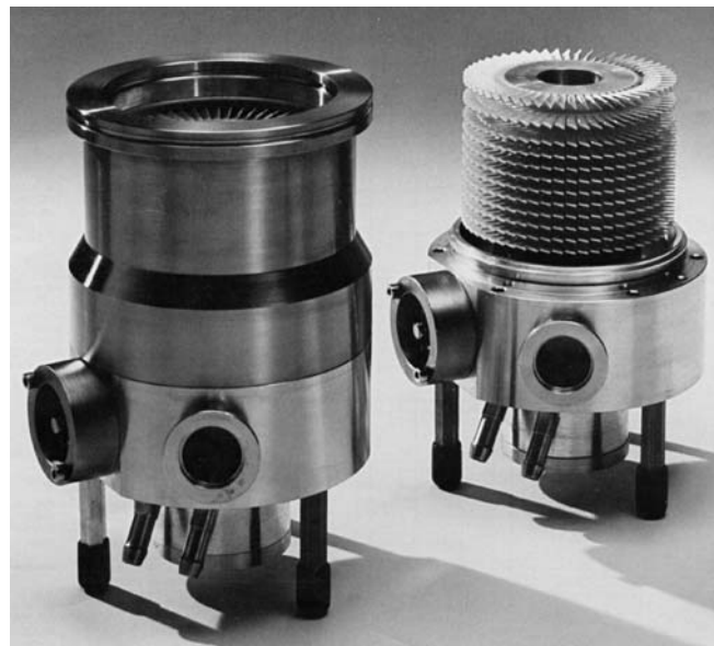
FIGURE 8.3. A turbopump (with and without its casing), which is nothing more than a small turbine that rotates at high speed. Like a jet turbine it pulls air in at the front end and forces it out of the back. The blades are designed like airfoils to enhance the flow of gas through the system.
