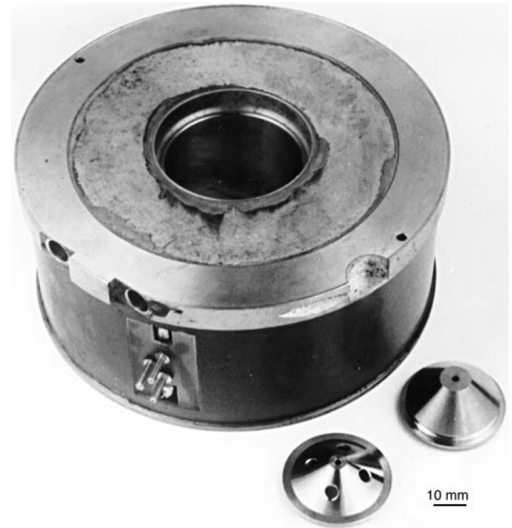
FIGURE 6.7. A real lens: the cylindrical shape conceals the copper wire coils. The two conical polepieces beside the lens sit inside the central hole in the lens. The three-pin electrical connections provide current to the coil to magnetize the polepieces, and cooling water is circulated in and out of the two holes in the top plate of the lens to dissipate the resistive heat generated in the coils. Compare this picture with the schematic in Figure 6.6.
