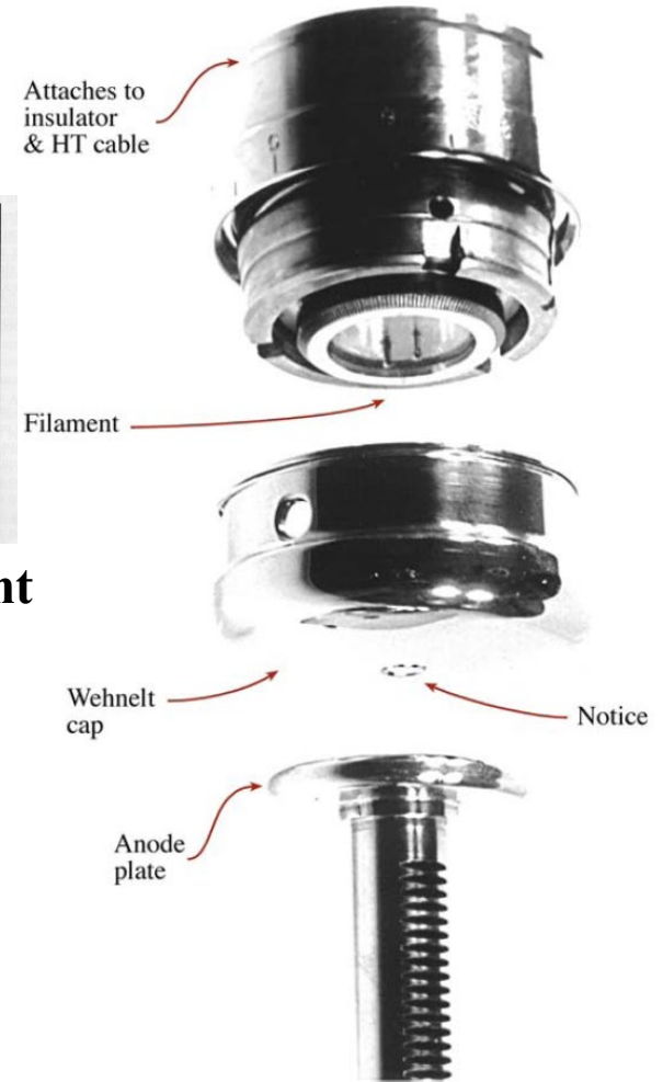
FIGURE 5.2. The three major parts of a thermionic gun, from top to bottom: the cathode, the Wehnelt cylinder and the anode shown separated. The Wehnelt screws into the cathode support and both are attached to the high-voltage cable which also contains power supplies for heating the cathode and biasing the Wehnelt. The anode sits just below the Wehnelt and the whole assembly sits on the top of the column of lenses that make up the rest of the TEM.
