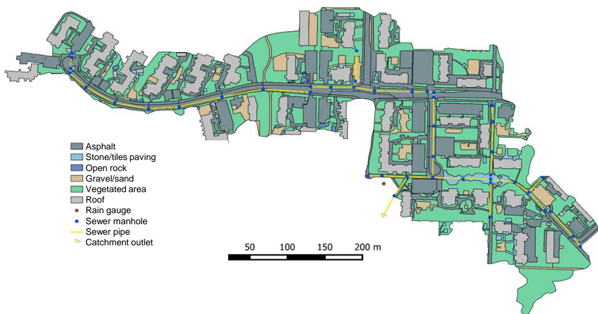
Figure 1. Surface types in Vallikallio and the locations of the sewer network and the catchment outlet. This map was obtained from the MSc thesis of Raudaskoski (2016) (available at: https://aaltodoc.aalto.fi/handle/123456789/19943 , in Finnish). More recently, Tuomela (2017) built a water quality model for the same study catchment (available at: https://aaltodoc.aalto.fi/handle/123456789/28476 , in English).
