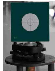
Targets for the registration of terrestrial laser scans
