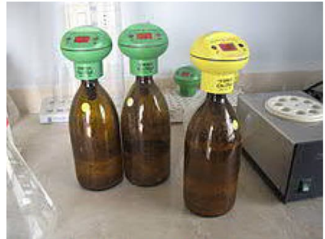
BOD test bottles at the laboratory of a wastewater treatment plant laboratory.
