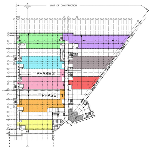
Figure 10: Location breakdown structure showing the “main bars” for Pentagon renovation (Figure 3 in Horman et al. 2003)
