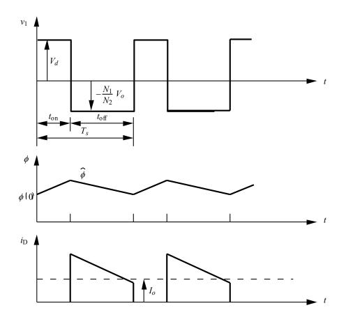
Peak value of the flux is at the end of conduction period
