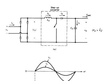
b) In PFC circuit input voltage and current can be assumed to be in phase
