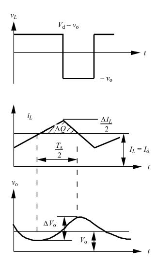
Inductor current and output voltage vaweforms are shown above. Output voltage change can be calculated from the change in charge,  $\Delta Q$ . Based on the area of the triangle
