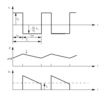
Peak value of the flux is at the end of conduction period
