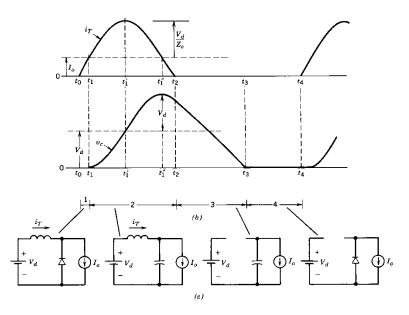
At time  $t_0$  switch is closed and input voltage  $U_d$  is over inductor  $L_r$  and its current increases linearly
