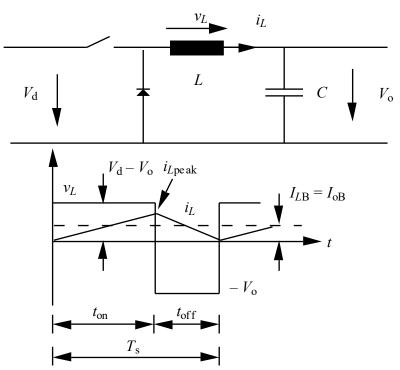
Waveforms in the borderline between CCM and DCM are shown above. Inductor current is derived form
