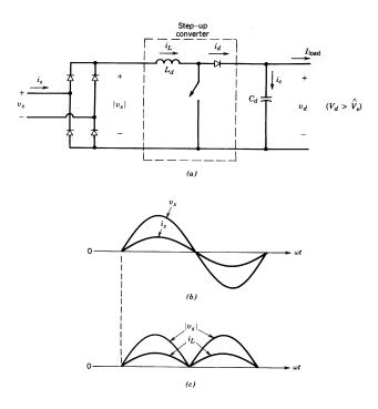
b) In PFC circuit input voltage and current can be assumed to be in phase
