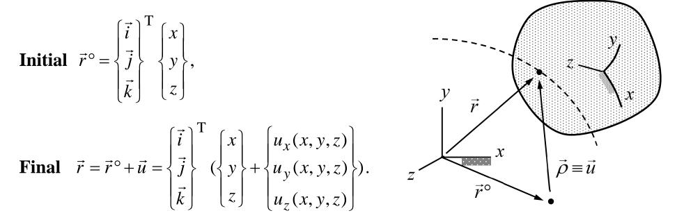
Displacement  $\vec{u}(x, y, z)$  is the primary unknown of a linear elasticity problem and other quantities like strain and stress are (finally) expressed in terms of it.
