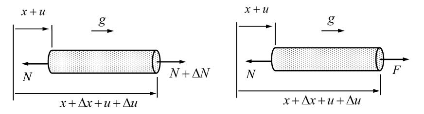
The cases where the material element is inside the bar and at the right end differ.
