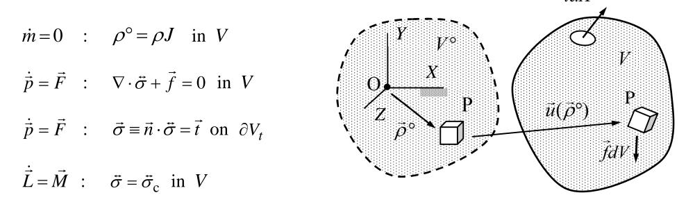
Assuming an equilibrium setting (geometry, stress, loading etc.) the local forms can be used used to find a new equilibrium setting (actually, displacements of the particles) when, e.g., external given forces are changed in some manner.
