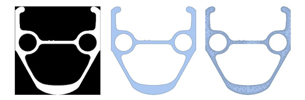
Triangle representation based on a picture from <u>www.mavic.com</u> the and cross-section moment definitions: R = 306 mm and  $I_{zz} = \sum_{e} \int_{\Omega^{e}} y^{2} dA = 3011 \text{ mm}^{4}$ .
