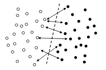
The ratio  $\Delta \vec{F} / \Delta A$  of the interaction force resultant  $\Delta \vec{F}$  to the area of the interaction  $\Delta A$  is assumed to be constant  $\vec{\sigma}$ , when the area *is not too small nor too large*, therefore also  $\Delta \vec{F} = \vec{\sigma} \Delta A$ . Although a certain range of lower and upper limits is involved, continuum mechanics uses the relationship in form  $d\vec{F} = \vec{\sigma} dA$ .
