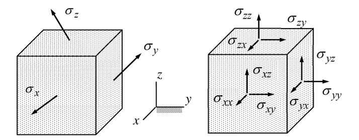
The first index of a stress component refers to the direction of the surface normal and the second that of the force component.
