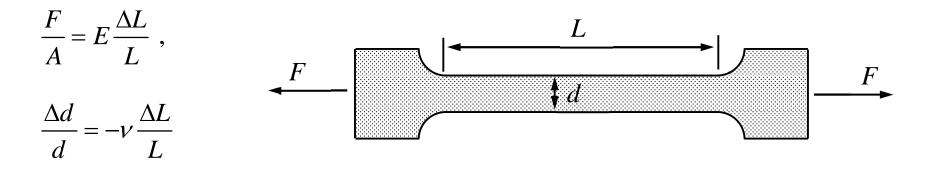
in which the coefficients E and v (Young's modulus and Poisson's ratio) depend on the material.
