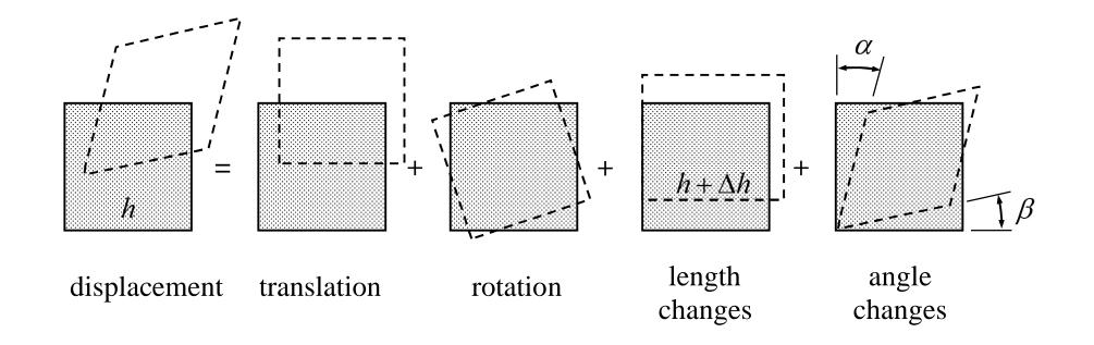
The geometry is described altogether by 12 parameters, of which 6 define the rigid body motion and remaining 6 the deformation (normal and shear components).
