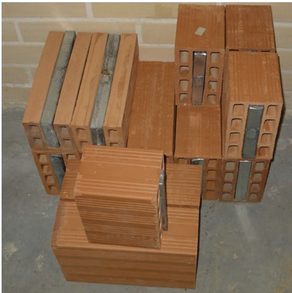
FIGURE 4.8 Clay bricks including PCM macrocapsules.
