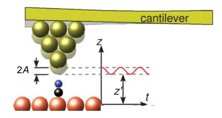
■ STM with an additional data channel giving the short-range tip-sample interaction
