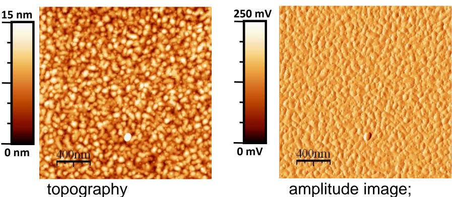
amplitude image; difference between the actual amplitude and the set-point
