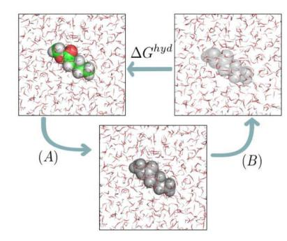
Thermodynamic cycle used to calculate solvation free energies. In the states of (*A*) the charge-charge interactions between the solute and its environment are progressively turned off (I scales interactions from 1 to 0). In states of (*B*), the dispersion interactions between solute and water are progressively turned off.
