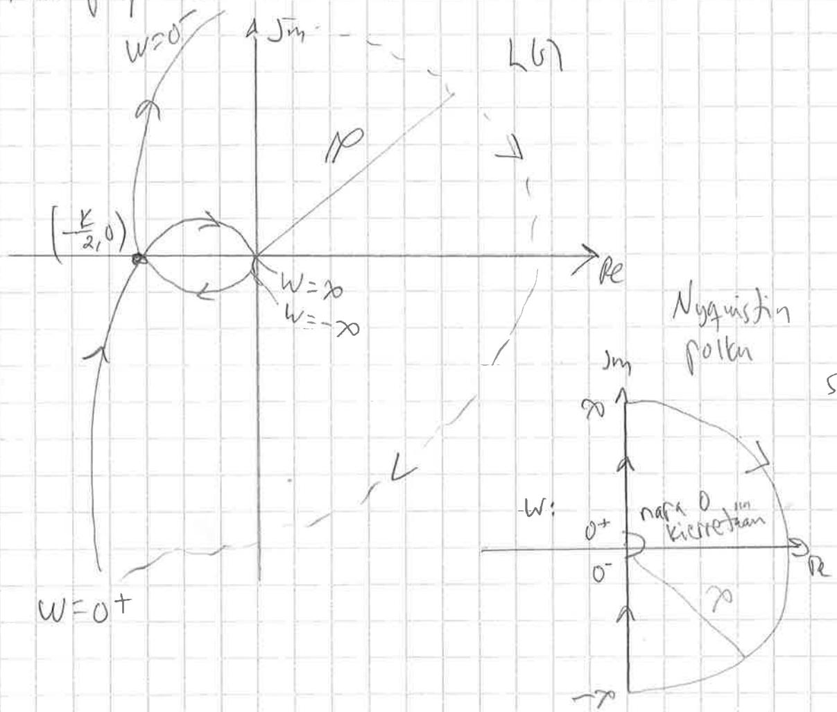
$$4. \quad G(s) = K \frac{\left(\frac{1}{\omega_0}s + 1\right)}{\frac{1}{K\omega_0}s + 1}, \quad G(j\omega) = K \frac{1 + j\frac{\omega}{\omega_0}}{1 + j\frac{\omega}{K\omega_0}}$$
