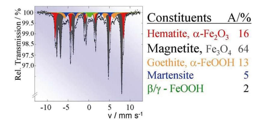
Routine Mössbauer analysis of finely dispersed corrosion particles formed in the cooling system of a power plant
