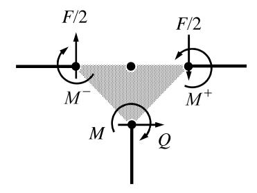
The shear forces and bending moments acting on a typical weld of size  $r \le h/2$  result into the moment equilibrium
