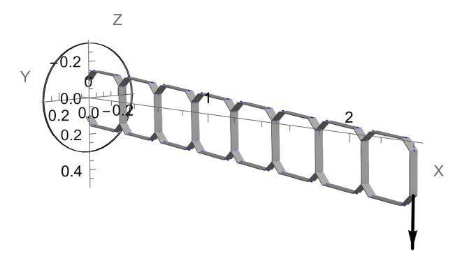
Numerical method is just a way to produce displacement-force data for given values of the problem parameters. For example, studying the effect of n means using the method with several selections of n. Table 2 shows the outcome of a FEM simulation with axially inextensible beams.
