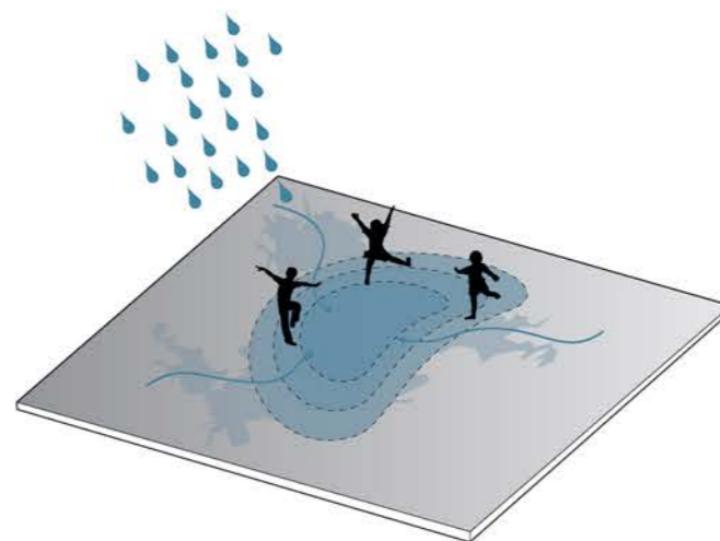
Subtle low zones in the paving, where rain water can gather.
