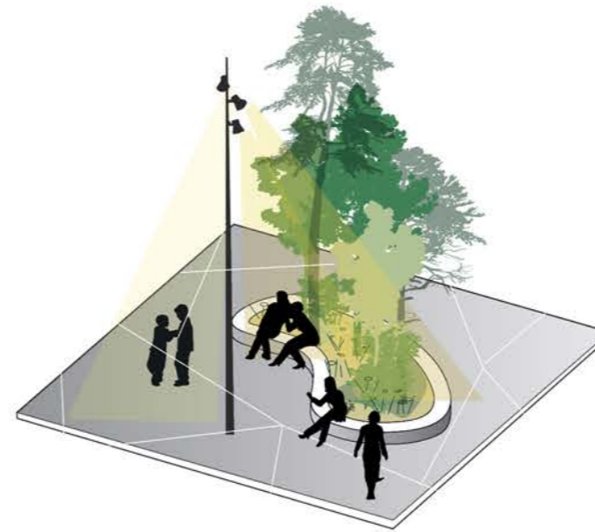
Higher lighting masts for overall good light conditions.
