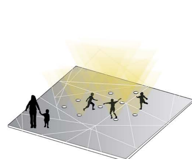
Uplights in the pavement for way-finding and accent.
