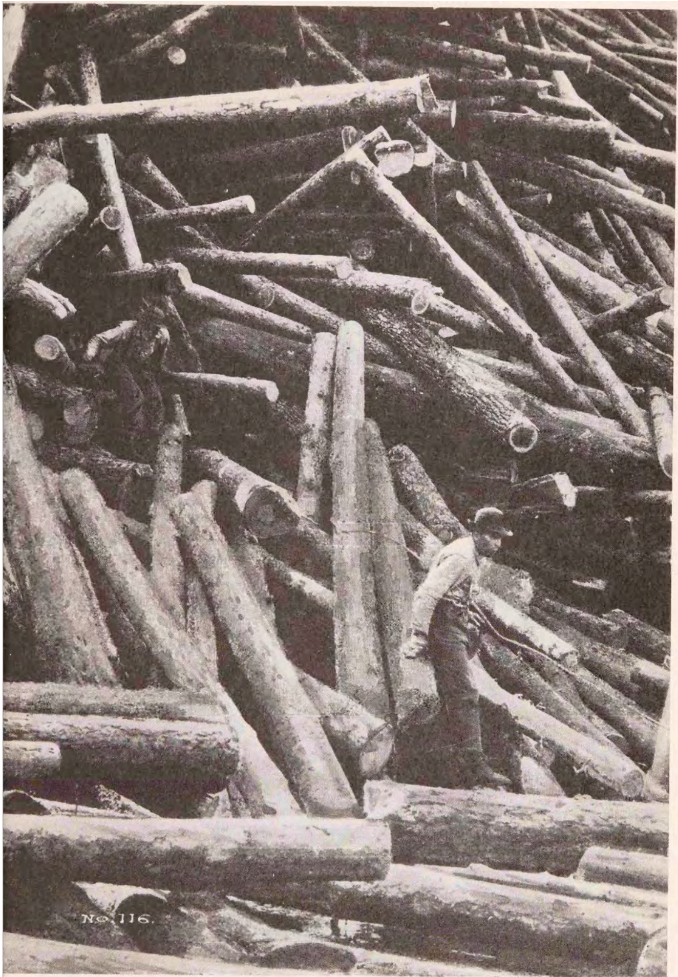
Breaking a jam. A logjam could be broken by using teams of horses to pull logs onto the shore, or even by dynamiting strategic logs in the hope of loosening the rest. But in the end, workers often had to go out onto the face and hack away by hand at the roaring mass. It was not a job for the faint of heart. Courtesy State Historical Society of Wisconsin.
