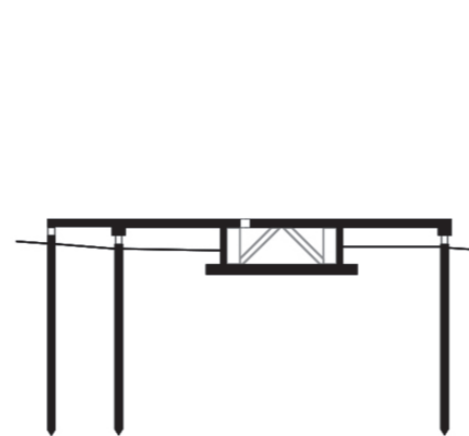
Construction foundations Wooden foundations -larch piles -technical gallery -grid of distribution
