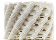
ceramic, 12 extruded ribs, 30°
