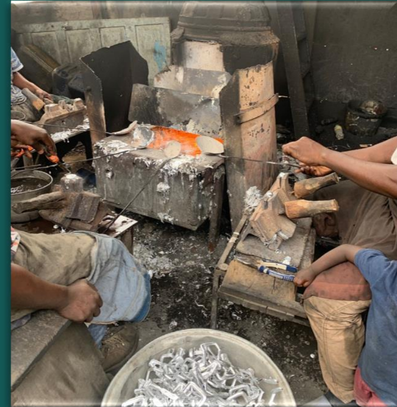
Images showing the firing of the ladles by workers
