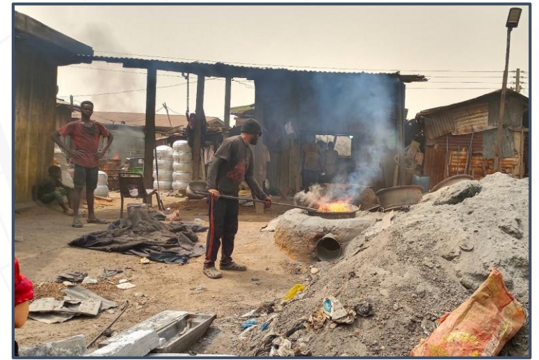
Melted down metal waste being used to create traditional pots and pans for . Source: Urban Field Study - 2023
