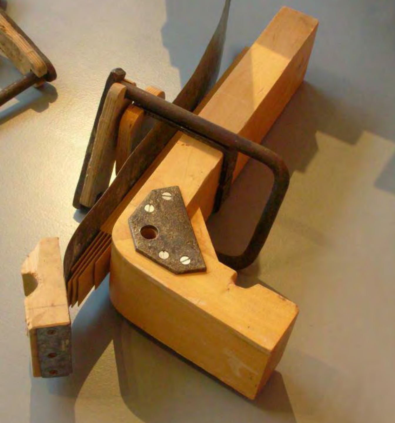
Formwork for the curved and birch leg laminated - Stool 60
