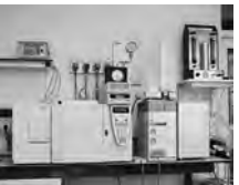
10 The analytical equipment: thermal desorption-gas chromatography-mass spectrometer
