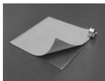
6 Mount the specimen on an inert support; seal the edges with aluminium tape
