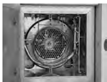
11 The separation process of the complex mixture takes place in the (brown) gas chromatography column
