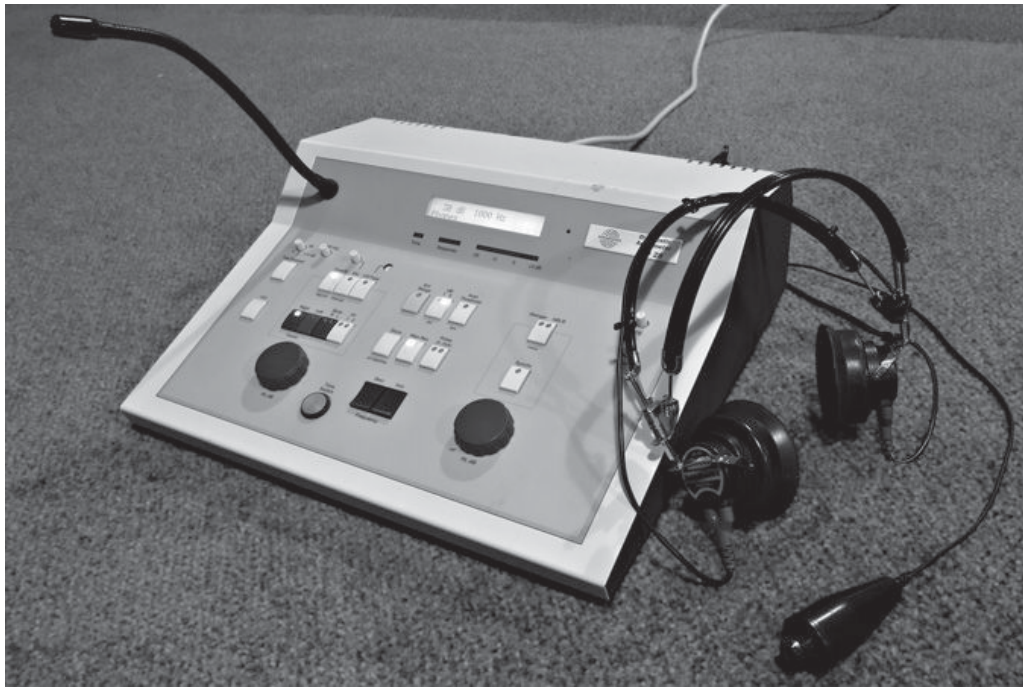
Figure 19.6 An audiometer with audiometric headphones and a patient-response button. Courtesy of Teemu Koski.
