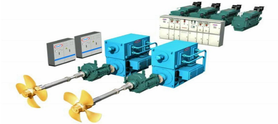
Figure 27 Example of Diesel-electric propulsion system (Ocean Time Marine, 2020)
