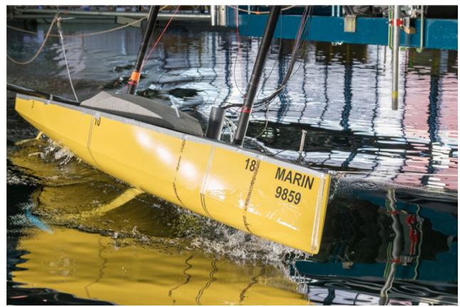
Figure 11: Picture of the VO65 model free running in bow quartering waves
