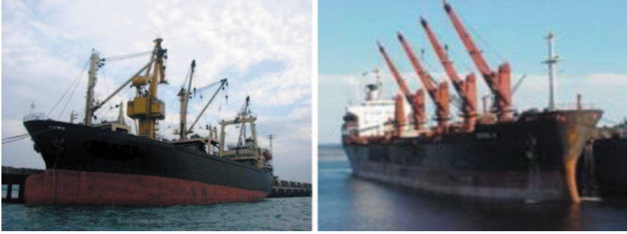
Fig. 2.87 Outdated and contemporary general cargo ships equipped with conventional derricks ( left ) and turning cranes ( right ) respectively
