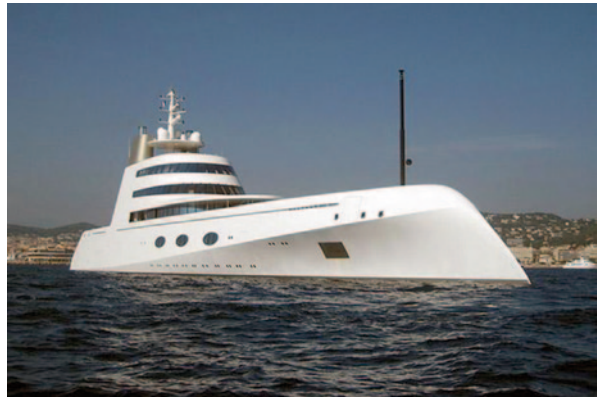
Fig. 3.34 Contemporary super luxury mega-yacht SIGMA A, shipyard Blohm and Voss (Germany 2008)—LOA 119 m, B 18.87 m, Tmax: 5.15 m, NPASS: 14, NCR: 37
