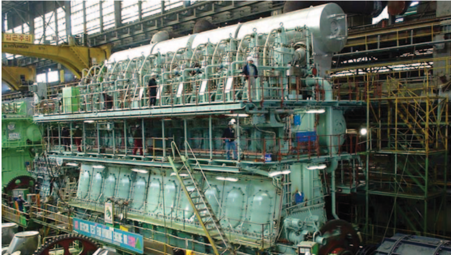
Fig. 5.6 Low-speed diesel engine MAN B&W 12K98MC (2004). 68,647 kW/93,360 PS, 94 rpm maximum. Heavy fuel oil: ISO-F-RMH, maximum viscosity 700 cSt. Consumption: 230 t/day for a 25-knot post-Panamax container ship
