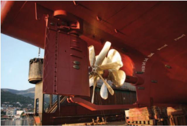
Fig. 5.32 Installation of O. Grim's vane wheel. The vane wheel is a second propeller downstream of the main propeller, which runs freely without torque on the shaft . The inner part of the vane wheel, the impeller or turbine part , has a pitch such that the vane wheel is driven by the wake of the main propeller. The outer part of the blades of the vane wheel, the propeller part , has a different pitch, which causes the vane wheel to generate thrust of the main propeller. The concept was originally proposed and patented by the late Prof. Otto Grim (Hamburg) in the 1960s; it is also known as Grim'sche Leitrad . Vane wheels are subjected to strong fluctuations in loading and problems with the strength of the blades have been encountered frequently, which has led to limited applications in recent years, despite significant powering/fuel savings, when smoothly working.
