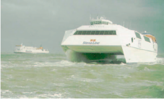
Fig. 2.78 All aluminum alloy high-speed hybrid SWATH HSS1500 of STENA Lines
