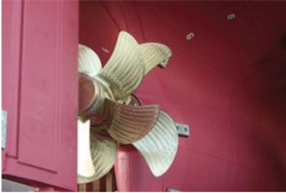
Fig. 5.31 Installation of co-axial contra-rotating propellers (CRP). The history of CRPs goes back to 1836, when a patent was filed by Ericsson applying it to a 45-foot ship. In 1909 and 1939, the Italian and US navies applied CRP to small steam powered ships. Since then, CRP has been widely used for torpedo propulsion, for small vessels and of course for prop aircraft propulsion; however, mechanical difficulties in producing reliable CR shafting, for large propulsive power have hindered in the past wide application to large merchant ships.
