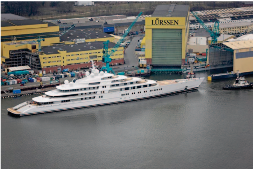
Fig. D.36 Largest superyacht in the world “AZZAM” ( L=180 m, V>30 knots, powered by a set of two gas turbines and two diesel engines with a total of 94,000 hp), launched in April 2013
