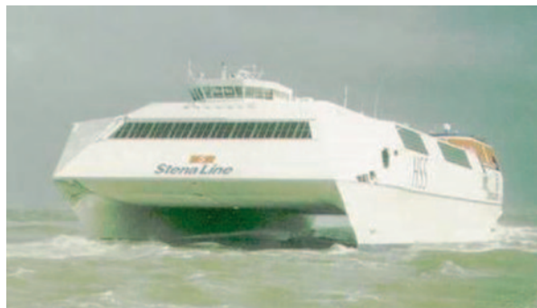
Fig. D.46 STENA’s HS1500 High-speed hybrid SWATH (built 1996 by Finnyards, all aluminum alloy LOA 126.6m twin hull construction, 1,500 passengers and 375 cars, trial speed 51 knots, service over 40 knots)
