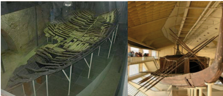
Fig. D.7 Kyrenia shipwreck and replica (Kyrenia castle museum, Cyprus) Ship sank in year 288 ( \pm 62 ) BC; it was discovered in year 1965; main ship dimensions 14 m length, 4.42 m wide, single square sail, 4–5 knots speed, 4 crew
