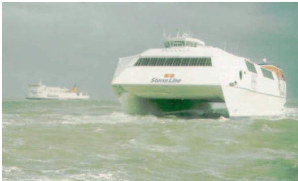
Fig. 1.31 High-speed catamaran of type SWATH ROPAX
