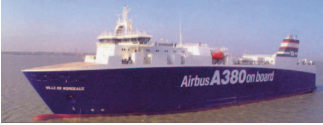
Fig. 1.27 RO-RO (Roll-On Roll-Off cargo ship)
