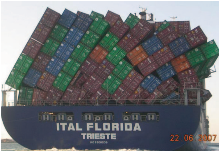
Fig. 2.96 Shift of deck containers due to excessive transverse accelerations
