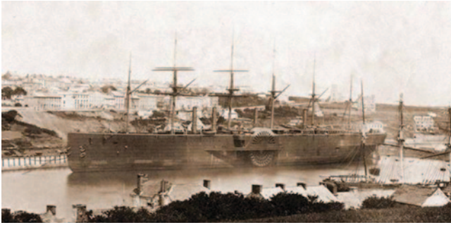
Fig. 5.12 SS Great Eastern (launched 1858), propelled by two side paddle wheels plus one screw propeller
