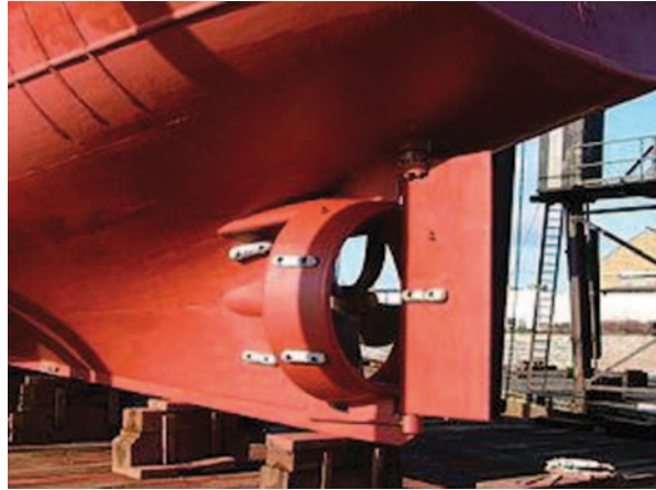
Fig. 5.19 Ludwig Kort's nozzle (invented 1934) and ducted propeller
