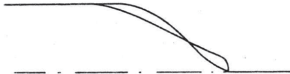
Fig. 3.52 Refinement of shoulders of sectional area curve of bulky ships with the application of a bulb
