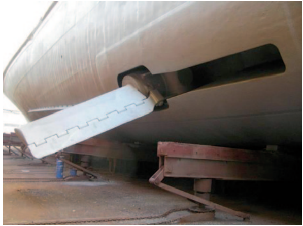
Fig. 2.53 Fin stabilizer on a cruise ship
