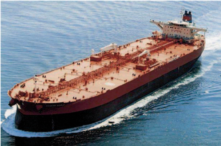
Fig. 3.60 Example of parabolic bow on tanker
