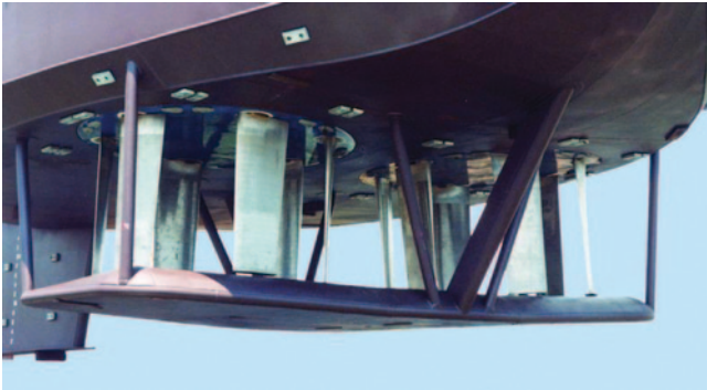
Fig. 5.29 Installation of Voith–Schneider propulsion system. The Voith–Schneider propeller was originally a design for a hydroelectric turbine. Its Austrian inventor, Ernst Schneider, worked with Voith's subsidiary in St. Pölten to further develop this concept to practical applications. It was found that Schneider's concept worked well as a pump, but, also, by changing the orientation of the vertical blades, it could function as an efficient propeller (first ship prototype in 1928)
