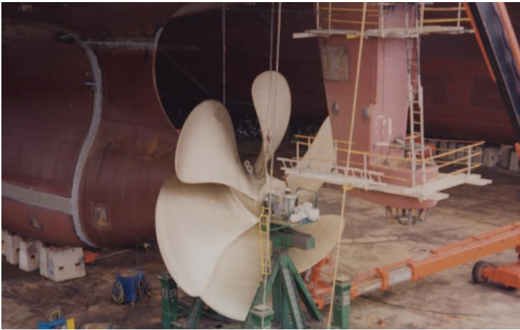
Fig. 5.14 Large, high powered, fixed-pitch propeller for post-Panamax container ship (2004). Diameter 9.10 m; six blades, total weight 102 t
