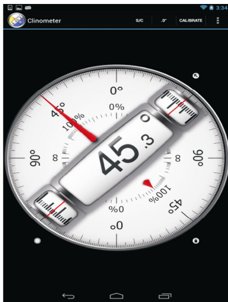
Fig. 9 Snapshot of the interface clinometer’s apps based on accelerometer sensor
