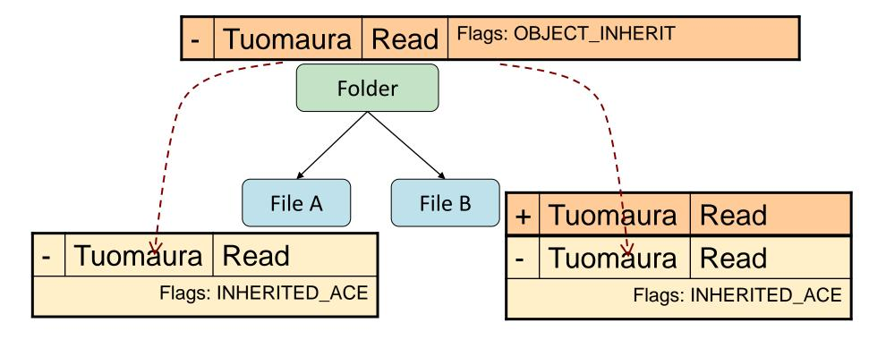
It is possible to override inherited negative ACEs because inherited ACES are placed at the end of the list
