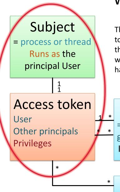
The process's access token is compared to the object's DACL when creating a handle to the object.
