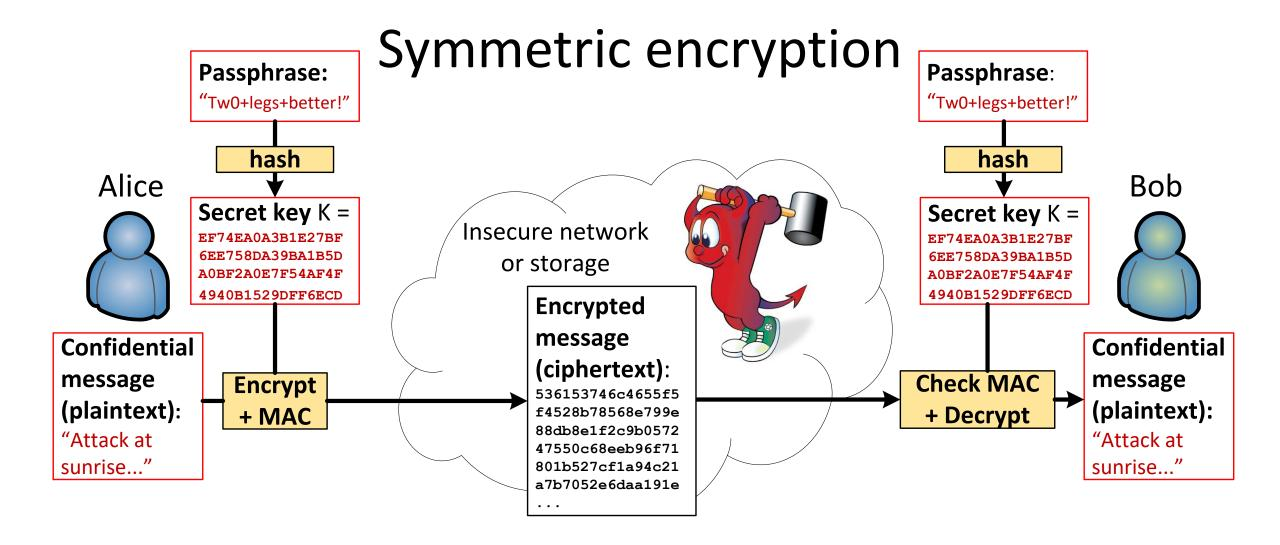
Message encryption based on symmetric cryptography,
