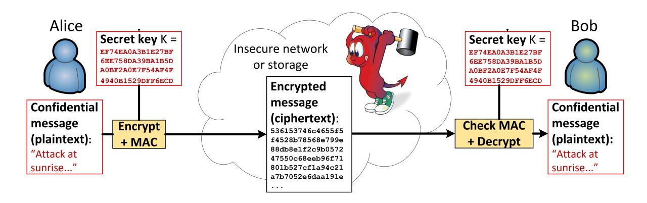
Message encryption based on symmetric cryptography,
