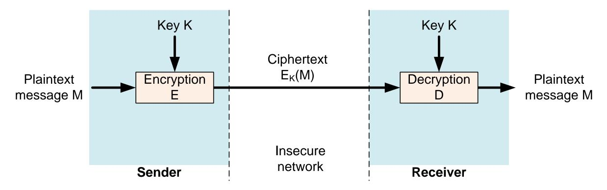
Message encryption based on symmetric cryptography,
