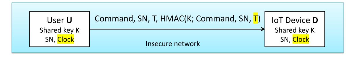
$U \rightarrow D$ : Command, SN, T, HMAC(K; Command, SN, T)
