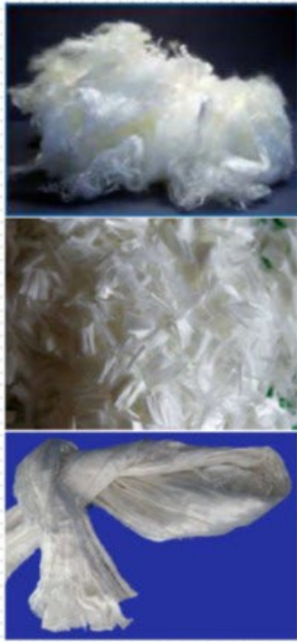
b) Titer (diameter): 0,5dtex–28dtex, (7–48µm) c) Fibre length: 3–120mm; endless tow
