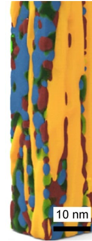
Electron tomography reconstruction of S 2 layer in spruce
